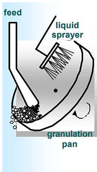
Fig. 1. Schematic of granulation processes (a) Traditional view (after Sastry and Fuerstenau [26]); (b) Modern approach [1].
